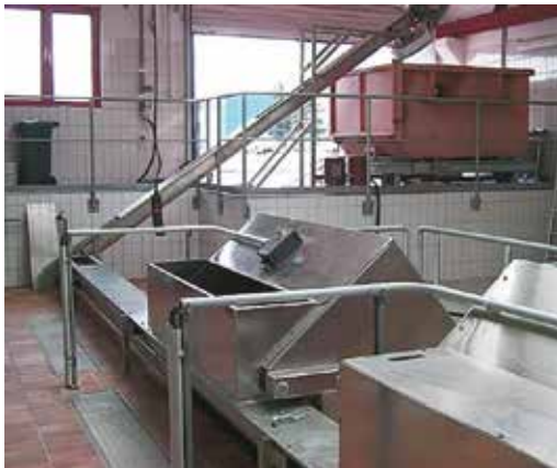
High accessibility guarantees easy maintenance and visual control of the screen
