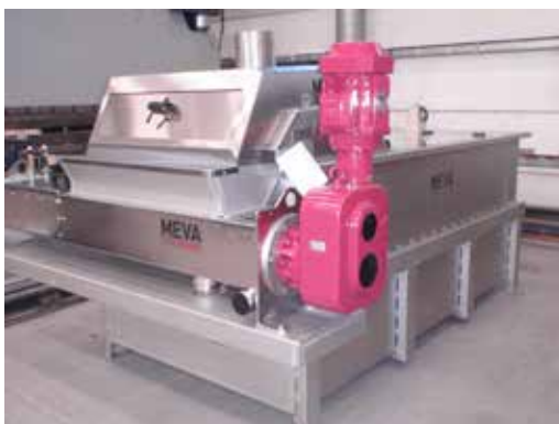
Meva Monoscreen mounted in tank with an SWP
