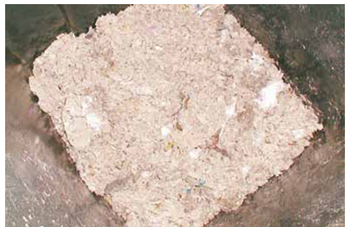
End product: washed, pressed and shredded screenings
